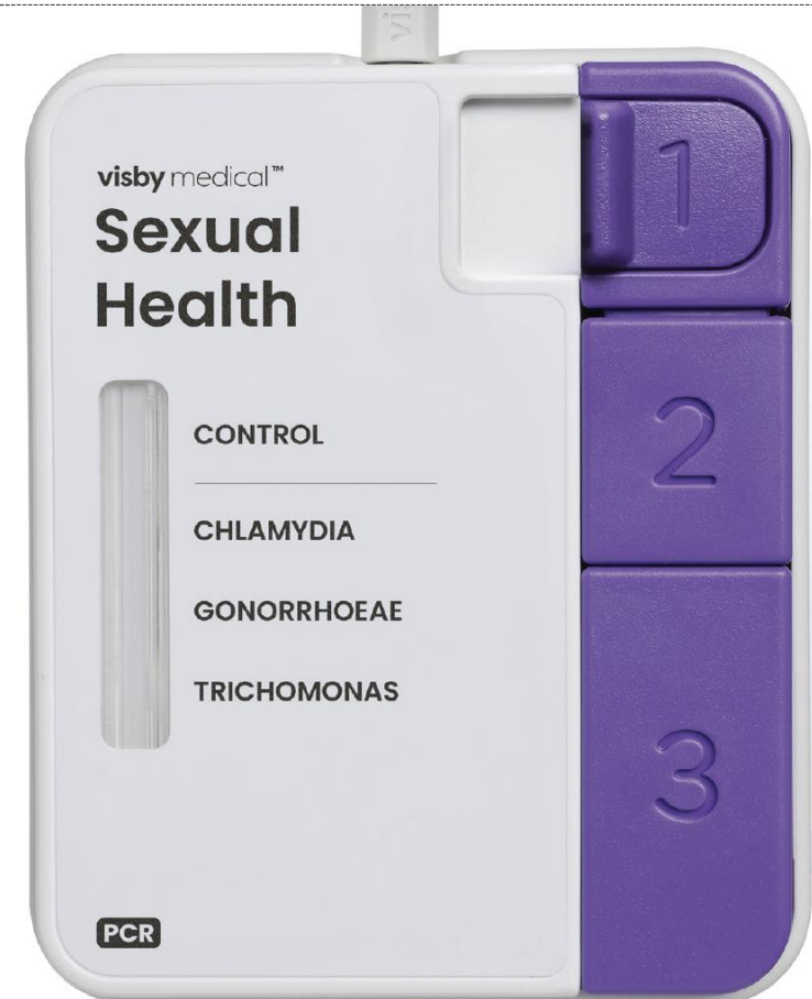
Morris, et al. Evaluation of the Performance of a single-use, rapid, point-of-care PCR device for the detection of Neisseria gonorrhoeae , Chlamydia trachomatis , and Trichomonas vaginalis : a cross-sectional study. Lancet ID .
